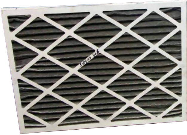
Actual 1 week old filter with old system
