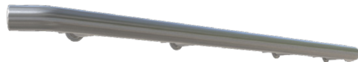
Cylindrical Continuous 1 1½" cylindrical handrail is a continuous metal form with ends turned toward the wall. We also offer straight endcaps in lieu of the returned ends. Comes in brushed stainless steel.
