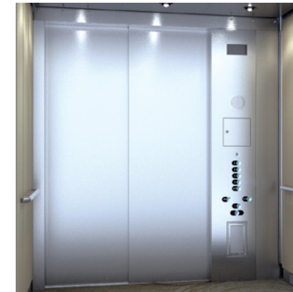
Two-speed door Provides a wider opening without compromising door cycling time. Two doors move in the same direction, one sliding faster than the other. Available with either right- or left-hand opening.
