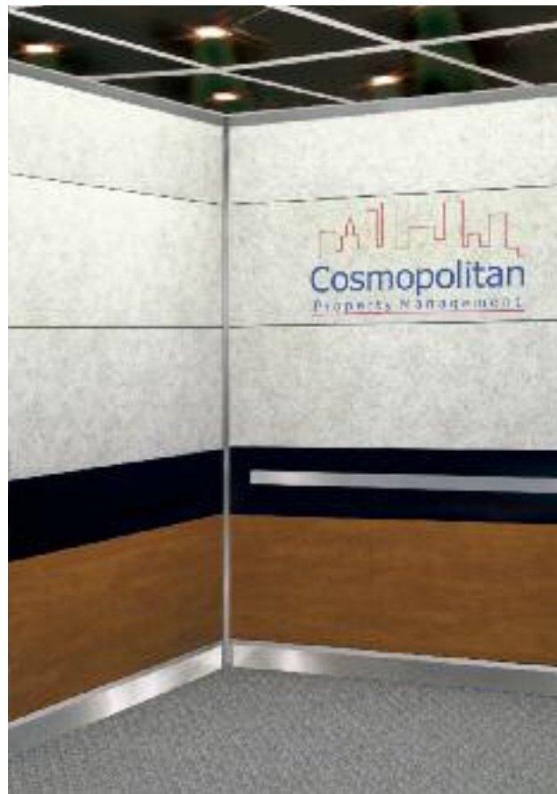
Impression II: layer 2 in Wild Cherry laminate; layer 3 in Black laminate; layer 4, 5 & 6 in Nirvana laminate with custom logo on back wall layer 5; Modular Downlight ceiling in Glossy Black laminate; 2" flat handrail
